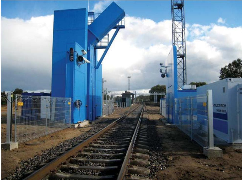
7.82 A further example of a Nuctech scanner with an energy level ranging from 1.5MeV to 6MeV that is used for "inspecting cars, cargo containers, empty containers, container trucks at seaports, border crossings, airports" is shown below<sup>98</sup>:
